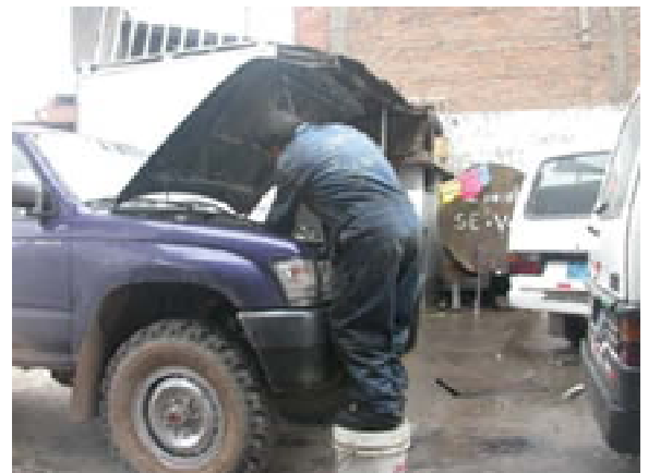
Mechanic in La Oroya converting the air and fuel mixture of the Hi-Lux for high elevations.
